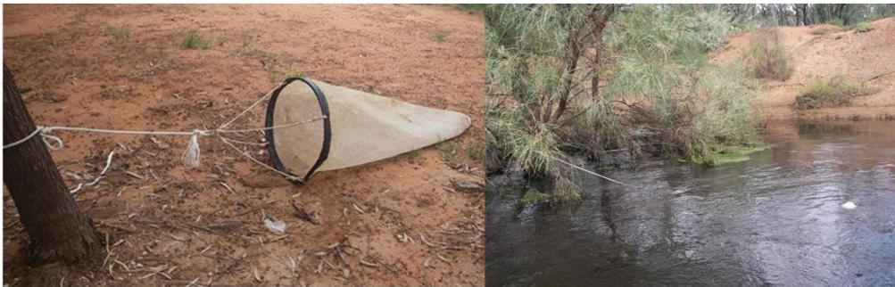
Figure 4. Drift net used in Murray River sampling adjacent to Margooya Lagoon.
