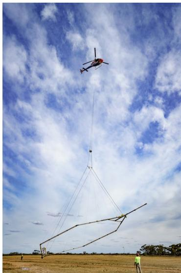
**Above:** The Mallee Salinity Survey is being undertaken by a low-flying helicopter equipped with a transmitter and receiver coil underneath it.
