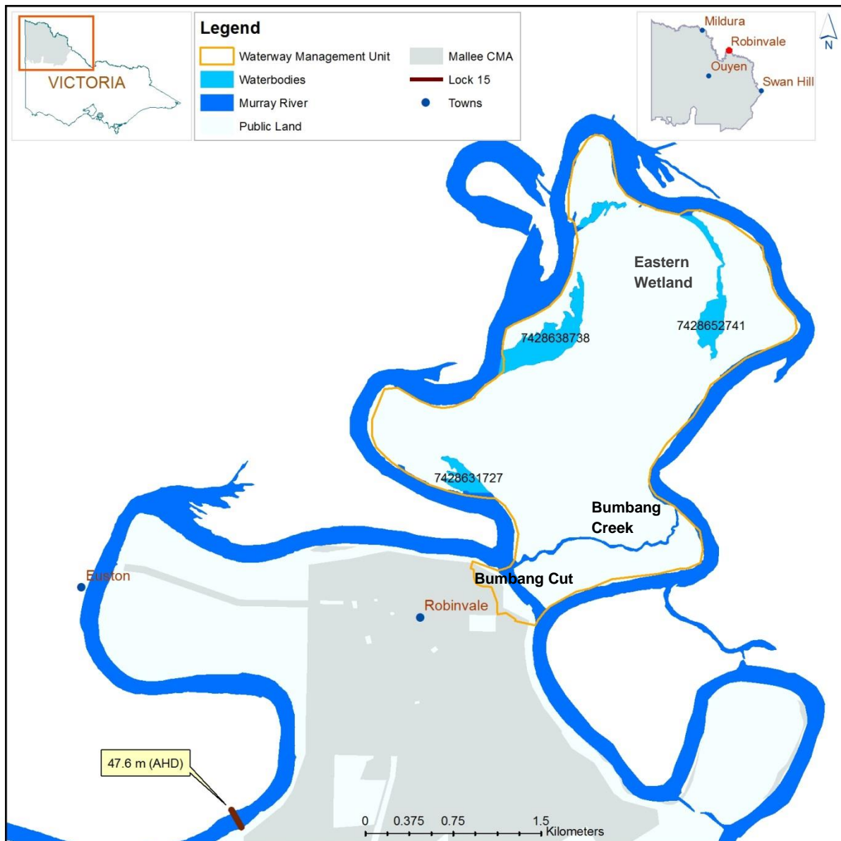
Figure 23. Approximate inundation extent of weir pool at 47.6 m AHD (0 m variation from normal operational height), inundating around 39 ha.
