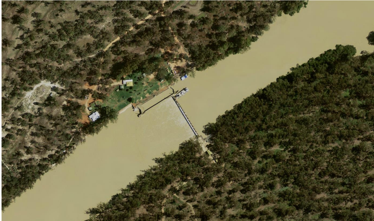
Figure 31. Lock 8 showing the lock on the north (right) bank. The fishway is on the south (left) bank (Source: Google Maps)
