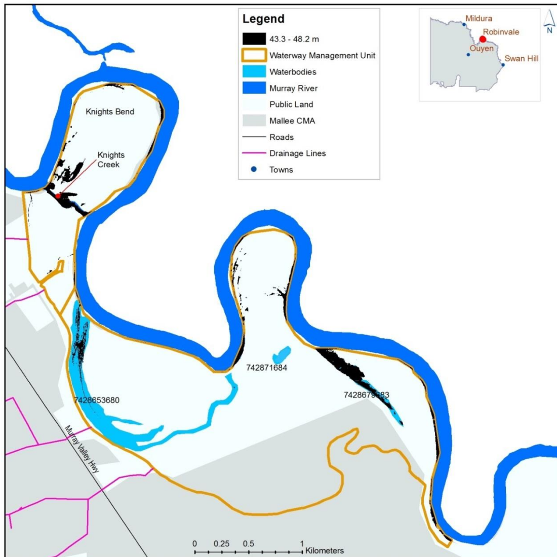
Figure 6 - Areas of Walshes Bend inundated at stable weir level 48.2m AHD (+0.6m above full supply level is shown in black). Inundation area estimated using LiDAR provided by Mallee CMA.
